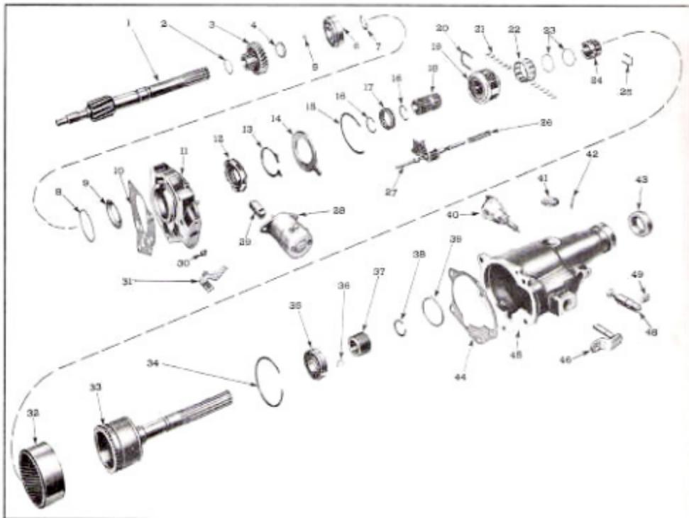
Fig. 40—Layout of Overdrive Parts
